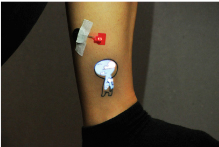
Fig. 1. Experiment in projection mapping: software developed in the Processing environment is used to track the position of a red led and use it as a reference to place a projected image precisely on the skin.
