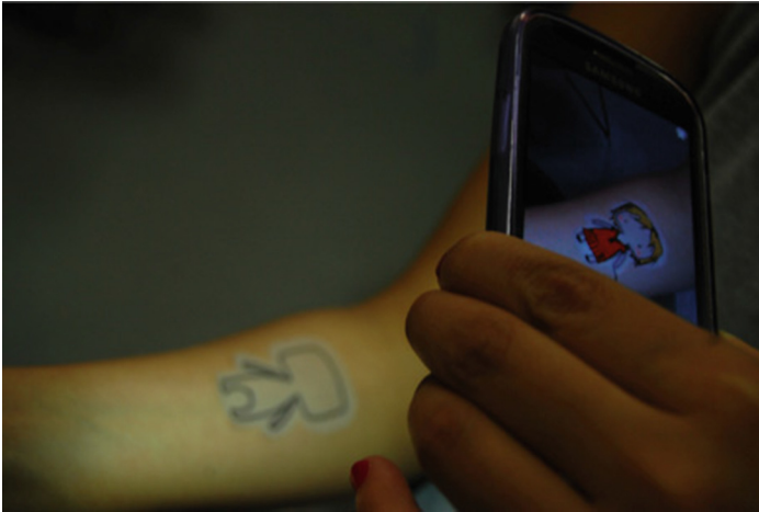
Fig. 3. A virtual image is positioned precisely over a drawing on the person's skin. In this experiment, a pen drawing over tracing paper was positioned on the user's arm and used as a tracking reference.
